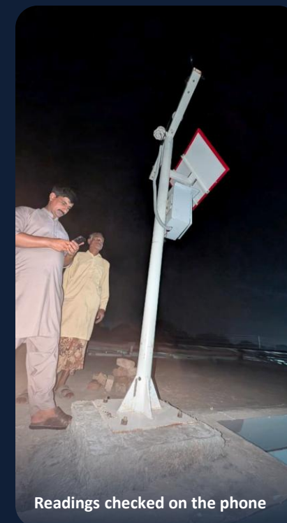
Solar panel, enclosure & sensor arm
